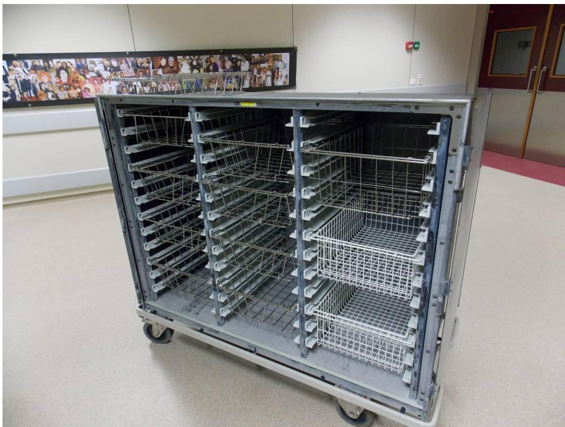
Figure 5: example of an external transport system used to contain individual sterile pack/trays in carrier baskets (as Figure 4).
