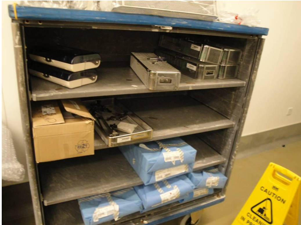
Figure 1: a transport cart showing signs of ageing with rough internal surfaces that may tear wrap when loading/unloading wrapped sterile packs/trays.
