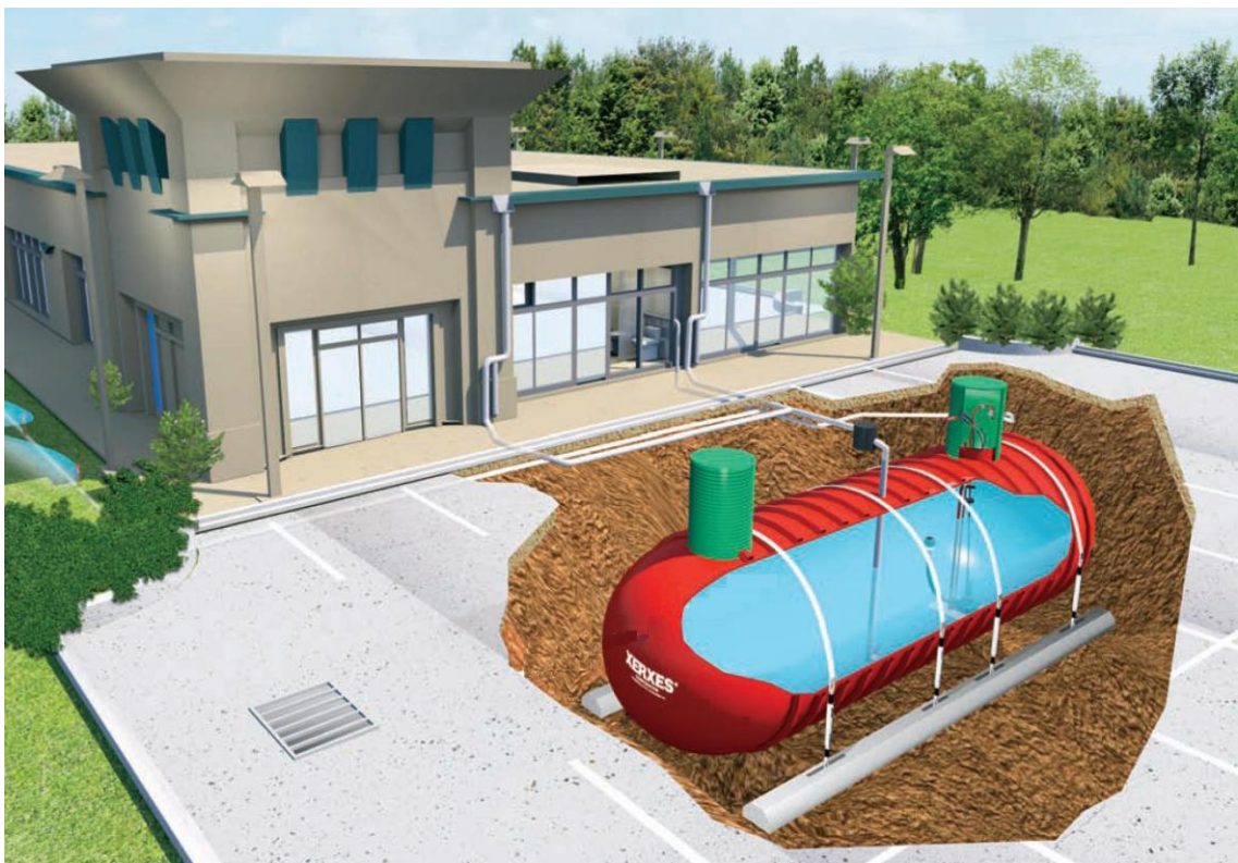
Figure 2: Typical rainwater harvester installation. (Source: http://capitolgreenroofs.groupsites.com/discussion/topic/show/48709.html?page=2 )
