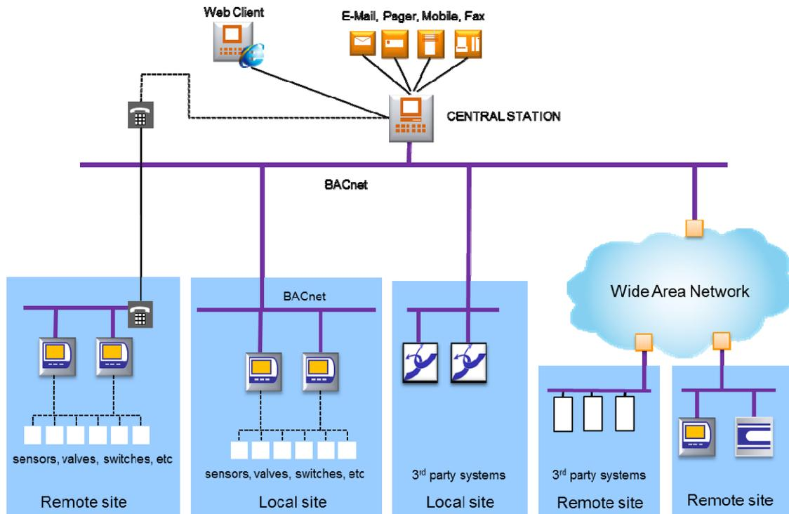
Figure 1: Building management system with remote access schematic
