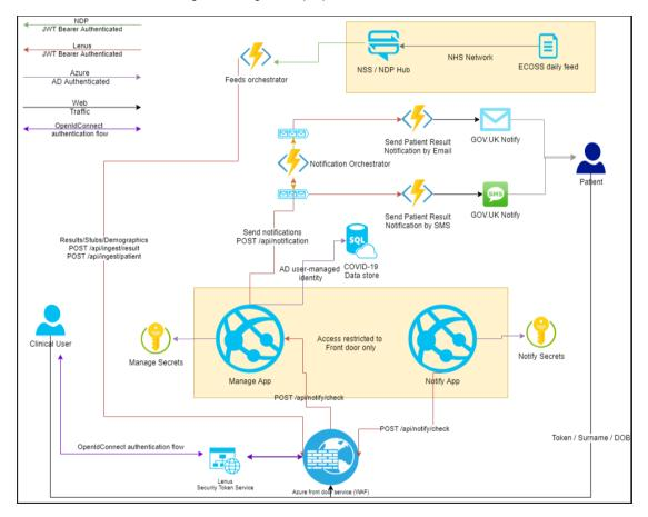
Figure 1: diagram of proposed architecture
