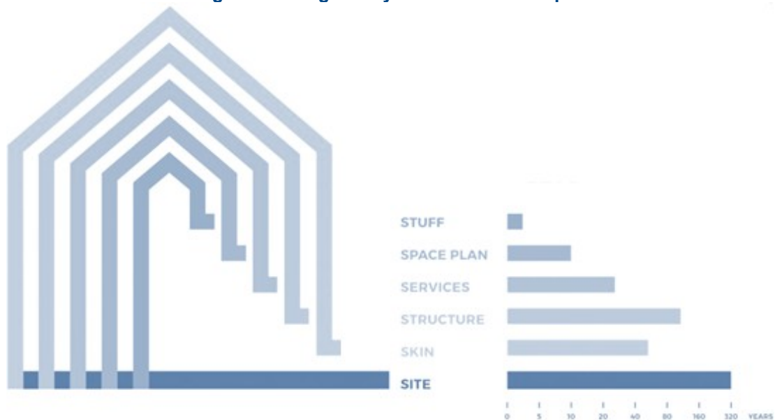
Figure 6: Design in layers – element lifespan
