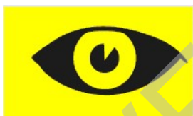
Figure 68: A symbol of an eye, developed from the British Standard symbol, using solid areas of colour instead of lines, which may increase the viewing distance
