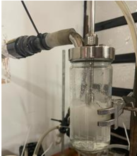
Figure 2: The suspension fluid in the Collison nebuliser.
