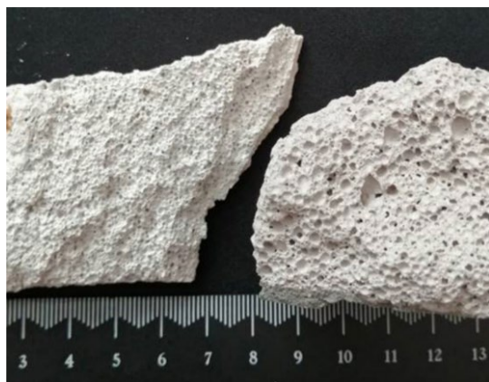
Figure 2.4 - Variability of AAC (page 4, 'Reinforced Autoclaved Aerated Concrete (RAAC) Panels Investigation and Assessment', IStructE, February 2022)
