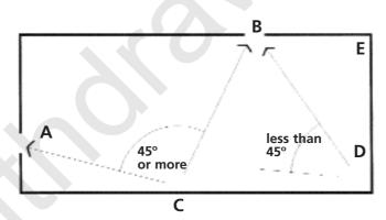
Provided that the maximum travel distance is less than 8 metres alternative escape routes are available from C because the angle ACB is more than 45°.
